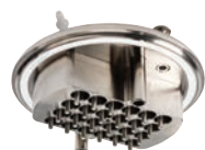
Combined reflux and additions head with nickel condensing fingers
